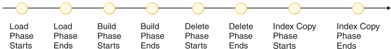
Figure 44. The Four Phases of the Load Process: Load, Build, Delete, and Index Copy
