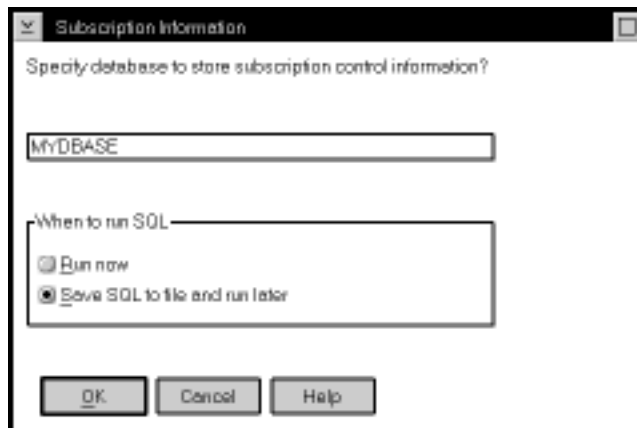
Figure 22. The Subscription Information Window. Use this window to enter the control server name and specify whether to run now or save the SQL to a file
