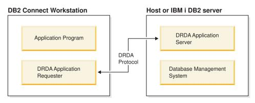
Figure 1. Data flow between a DB2 Connect server and an IBM mainframe server
