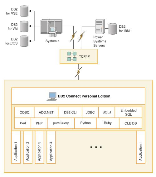
Figure 3. Direct Connection Between DB2 Connect and an IBM mainframe database server
