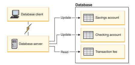
Figure 2. Using a Single Database in a Transaction
