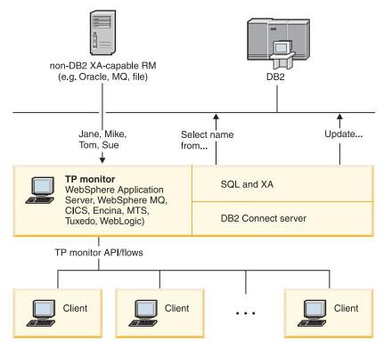
Figure 7. DB2 Connect support for TP monitors
