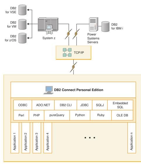
Figure 4. Direct connection between DB2 Connect and an IBM mainframe database server
