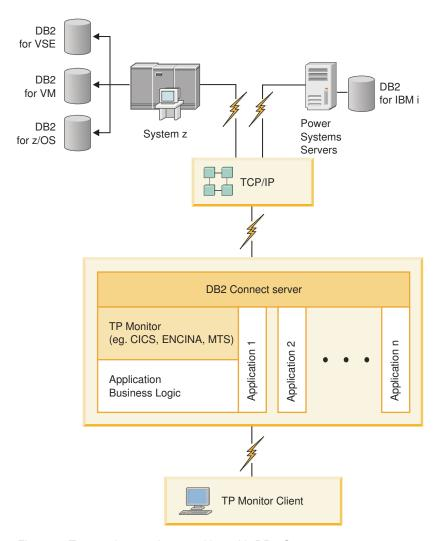
Figure 3. Transaction monitors working with DB2 Connect.
