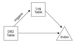
Figure 2. Incremental update process with triggers
