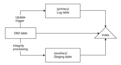
Figure 3. Incremental update with triggers and integrity processing
