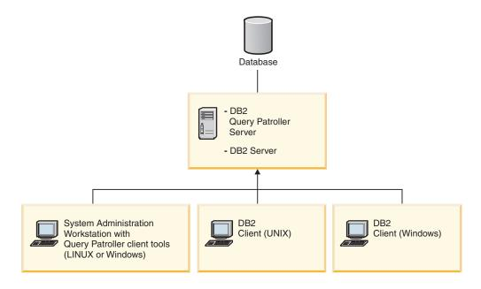
Figure 2. Query Patroller nonpartitioned database installation environment
