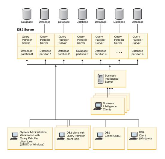
Figure 3. Query Patroller partitioned database installation environment
