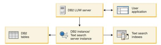
Figure 1. Deployment diagram for the DB2 Text Search server
