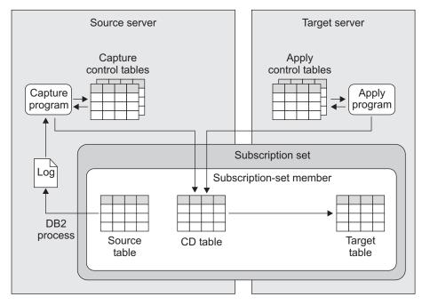
Figure 1. A simple configuration in SQL replication
