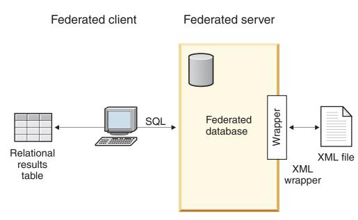
Figure 22. How the XML wrapper works
