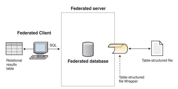
Figure 8. How the table-structured file wrapper works
