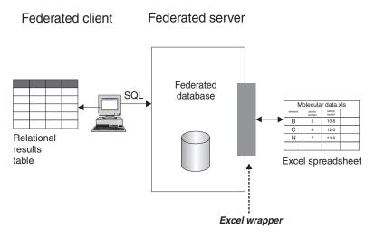
Figure 3. How the Excel wrapper works
