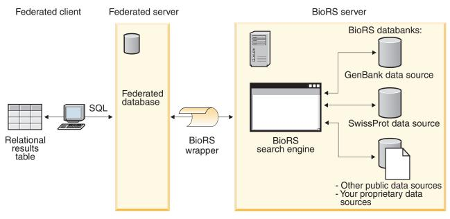
Figure 2. How the BioRS wrapper works
