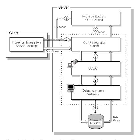
Figure 3-1: Hyperion Integration Server Components and Connections
