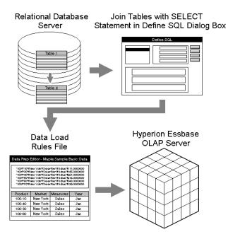
Figure 7: Loading SQL Data by Joining Tables in the Application Manager
