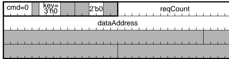
Figure 9-1 — OUTPUT_MORE command descriptor format
