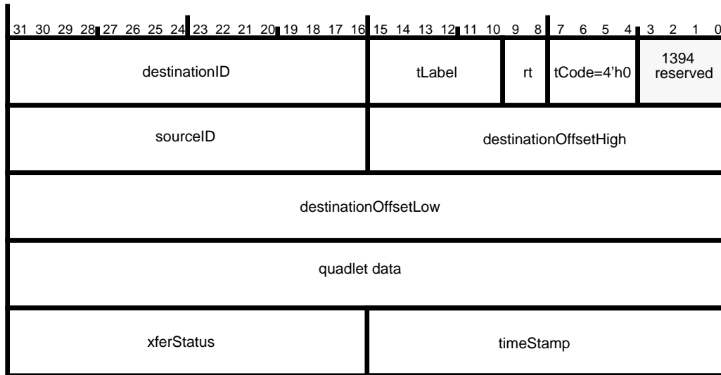
Figure 8-9 — Quadlet write request receive format
