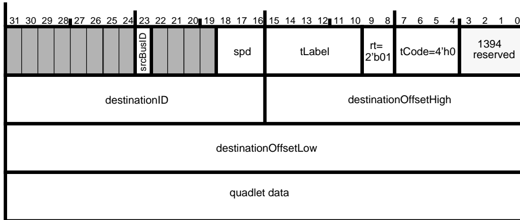
Figure 7-9 — Quadlet write request transmit format
