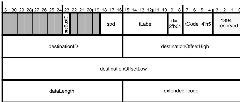
Figure 7-10 — Block read request transmit format
