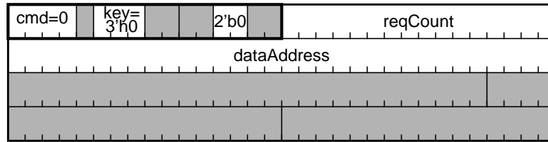
Figure 9-1 — OUTPUT_MORE command descriptor format
