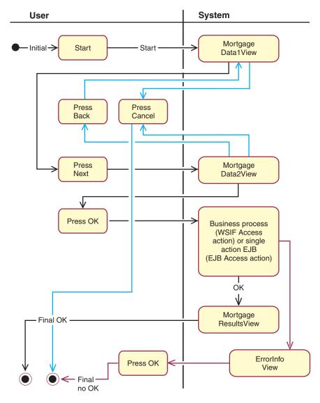
To use a flow processor in this way, a user externally defines the set of states of the process, along with their corresponding transitions (specific events fired by the visual components) and the actions (such as perform a business process in the application logic layer, start another processor implementing a subflow, and open another view) for the flow processor. In this way, the user does not hardcode the execution of specific actions into the views.
