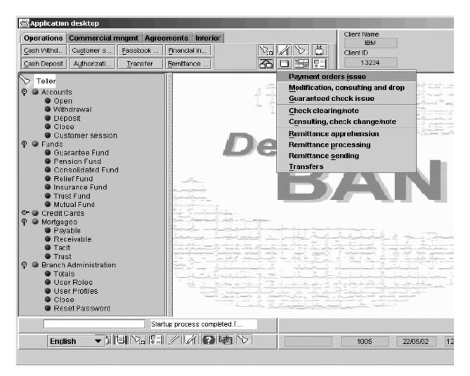
Some XML Desktop components implement the TaskLauncher interface, which the component uses to open a new task and display the initial panel for that task. The TaskLauncher associates the task with a single navigation flow, which steps the user through the different panels and executes the operations associated with the business process that the flow represents.
