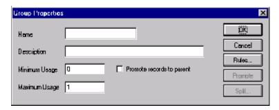
2. In the Name box, type "PODetailGroup" to indicate that this group contains all of the detail records. This is the segment loop identification code.
