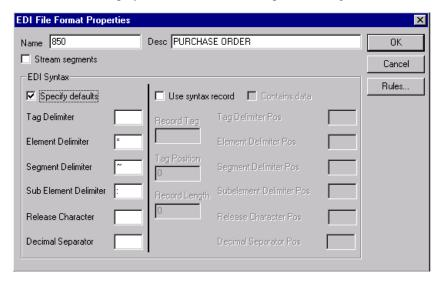
In the EDI Syntax section, verify that the Specify defaults check box is selected. 3. Verify the required delimiters for the ANSI X12 standard. If the delimiters differ from the default in the table below, type either the character or the hexadecimal value in the correct box. The default delimiters for ANSI X12 are the following (the tag delimiter, release character, and decimal separator are not used for ANSI):
