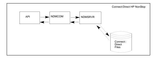
The following figure shows the flow of a request through Connect:Direct HP NonStop.
