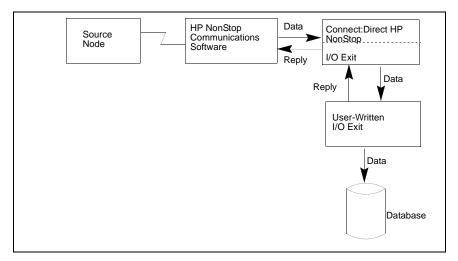
The following figure shows the data flow of a standard I/O exit on the sending side:
