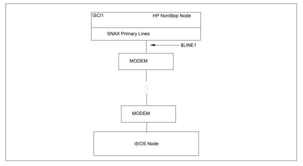
The SYSGEN and SCF definitions for receiving connectivity over SDLC switched lines follow. They define the HP NonStop node connected with a switched line connection to an i5/OS node with a synchronous communications board ready to dial in to the HP NonStop node.
