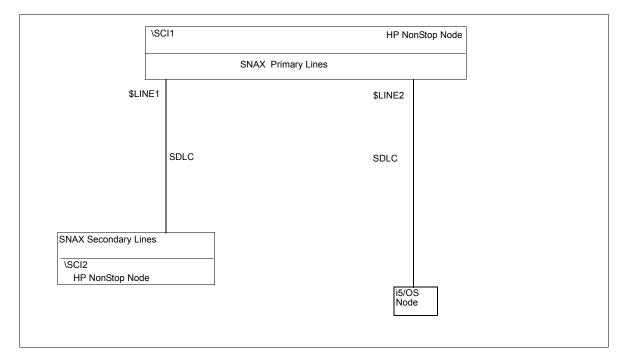
The SYSGEN and Subsystem Communication Facility (SCF) definitions for receiving connectivity over SDLC leased lines follow. They define the HP NonStop node connected to:
