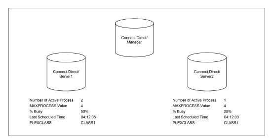
2. The Connect:Direct Manager receives a new Process. After determining that both Connect:Direct Servers support the PLEXCLASS required to run the Process, the Connect:Direct Manager determines which Connect:Direct Server has the lowest workload.
