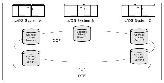
Connect:Direct/Plex operation is transparent; it appears as a single local node to other systems that communicate with it.
