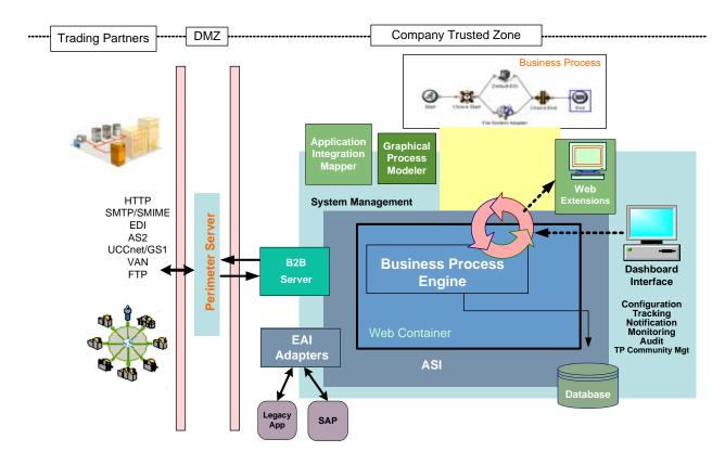
The following figure shows a simplified view of the system architecture:
