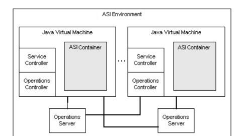
The following figure shows the service and operations controllers:
