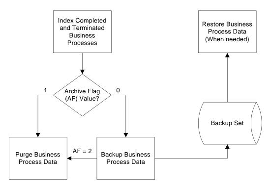
The Archive Flag is initially set by the Index Business Process service to 0 or 1. A value of 0 causes the data to be backed up. A value of 1 causes the data to be purged without being backed up. A data backup sets the flag to 2, which causes data to be purged.
