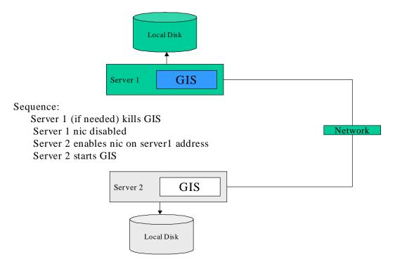
This option, with completely separate disk, is in may ways the simplest and cheapest way to go. It amounts to having two identically configured computers with Gentran Integration Suite installed identically on each.
