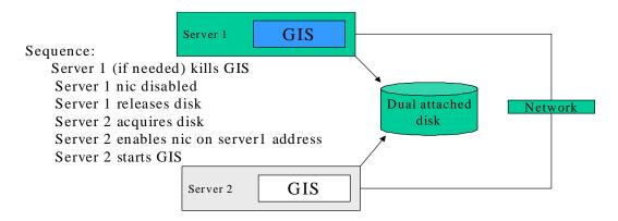
The objective is to take a standard Gentran Integration Suite installation on one node, detect failures, disable the first node, enable a second node, and start an identically configured Gentran Integration Suite. The exact mechanics of this process will vary, depending on the hardware and software involved.
