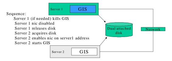
This option, using dual attached hardware, requires disks that have the capability of being attached to two (or more) servers. Most modern external storage subsystems can do this (with varying degrees of sophistication).
