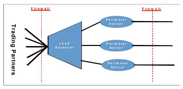
The following figure shows a typical configuration for perimeter server for high availability:
