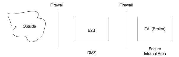
However, within Gentran Integration Suite it is more appropriate to view the B2B server as a complex adapter. The B2B server has a two-part Service Adapter Implementation. One part runs in the DMZ and one part runs in the ASI environment.
