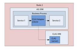
This diagram illustrates the process flow between the CLA2 adapter client and the CLA2 adapter server on different hosts with multiple CLA2 servers:
