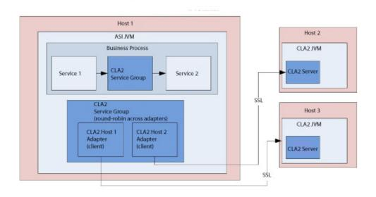
This diagram illustrates the process flow between the CLA2 adapter client and the CLA2 adapter server on different hosts that are secured with SSL:
