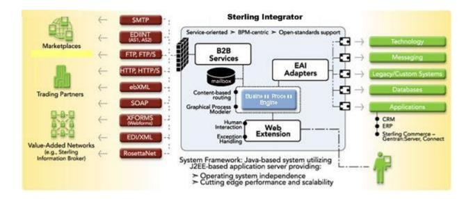
The figure depicts a Sterling Integrator system using many B2B services and EAI adapters. Your configuration will use only the services and adapters that are required for integration activities. The figure also shows a mail box component and integrated human interaction points through Web Extensions, which you may or may not decide to employ.
