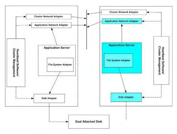
The shaded components would be disabled until the cluster manager determined that there had been a failure. At that point.
