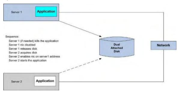
This option, using dual attached hardware, requires disks that have the capability of being attached to two (or more) servers. Most modern external storage subsystems can do this (with varying degrees of sophistication).
