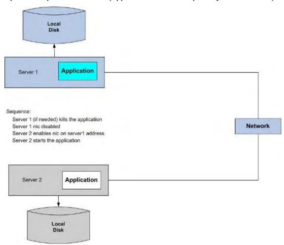
Option 1: Separate Local Disk (Application Installed Separately On Each Node)
