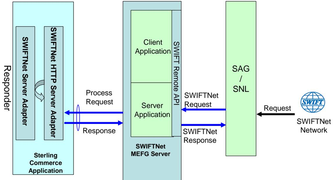
The SWIFTNet Client adapter (in conjunction with the SWIFTNet HTTP Server adapter) enables you to use Secure Sockets Layer (SSL) to provide secure authentication, using the SWIFTNet HTTP Server adapter to accept the forwarded request from the SWIFTNet MEFG Server. When you use SSL with Application, two channels are secured: an Outbound channel (Application acting as the Requestor) and an Inbound channel (Application acting as the Responder).
