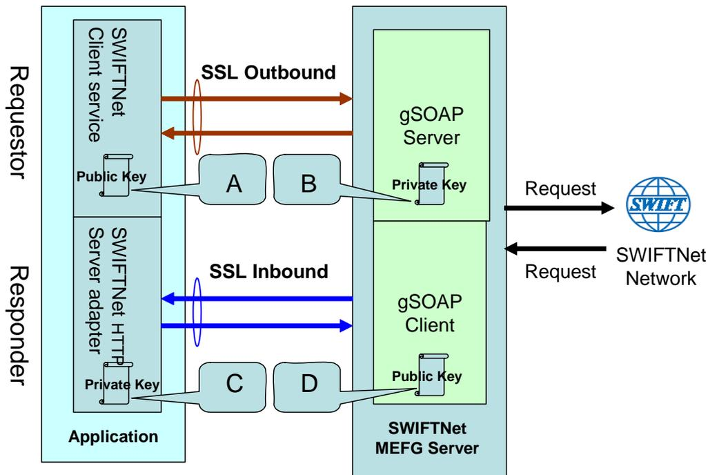
You will need 2 pairs of certificates. The first pair belongs to the SWIFTNet MEFG Server (A and B in the diagram above) and is used to secure the outbound channel. The second pair of certificates belongs to Application (C and D in the diagram above) and is used to secure the inbound channel. In the above diagram, the callouts signify the following:
