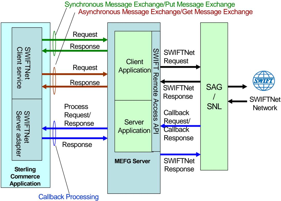
The SWIFTNet Server adapter (in conjunction with the SWIFTNet HTTP Server adapter) enables you to use Secure Sockets Layer (SSL) to provide secure authentication, using the SWIFTNet HTTP Server adapter to accept the forwarded request from the SWIFTNet MEFG Server. When you use SSL with the
