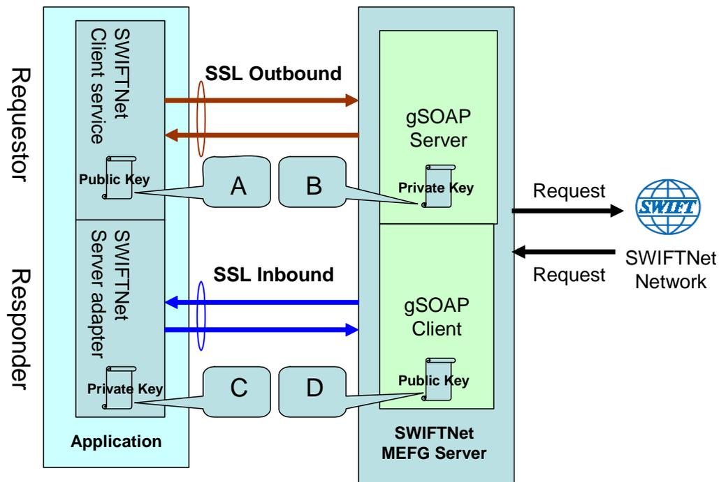
You will need 2 pairs of certificates. The first pair belongs to the SWIFTNet MEFG Server (A and B in the diagram above) and is used to secure the outbound channel. The second pair of certificates belongs to the application (C and D in the diagram above) and is used to secure the inbound channel. In the above diagram, the callouts signify the following:
