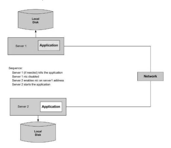
This option, with a completely separate disk, is in many ways the simplest and cheapest way to go. It amounts to having two identically configured computers with Sterling B2B Integrator installed identically on each.
