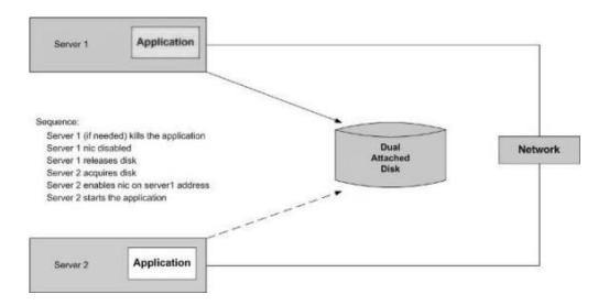
This option, using dual attached hardware, requires disks that have the capability of being attached to two (or more) servers. Most modern external storage subsystems can do this (with varying degrees of sophistication).
