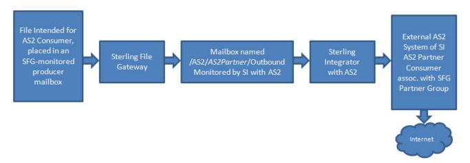
The following diagram shows the flow of inbound AS2 messages between Sterling File Gateway and other systems.
