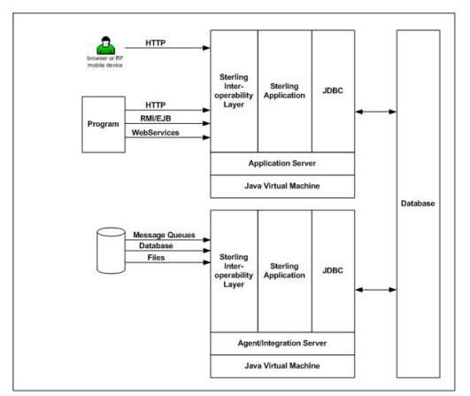
These components run inside a Java Virtual Machine (JVM). As a result, each component exists as a process in the system. You can have multiple instances of each component. For example, you can run Sterling Selling and Fulfillment Foundation in multiple instances of the application server. Each instance is a separate JVM.
