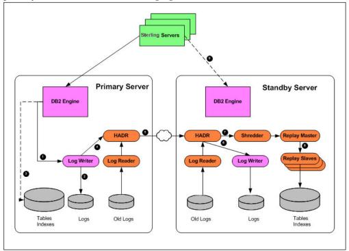
At a high level, the log writer on the primary database server records changes to its local transaction logs. These logs are critical for crash and instance recovery. The primary HADR sends the log records to the standby HADR where the logs are written out to the standby server's transaction logs. The changes are then applied to the standby server's database. At some point in time, the changes on the primary server are asynchronously written to the database.
