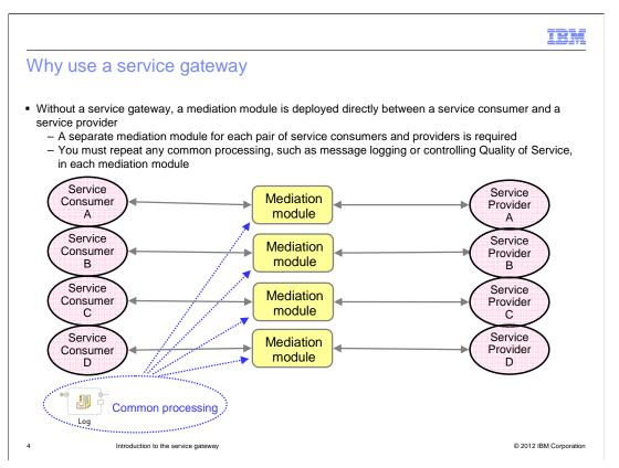
Here is a typical configuration when a service gateway is not used. In this case, a mediation module is typically deployed directly between a service consumer and a service provider. This means that you need a separate mediation module for each pair of service consumers and service providers. You must repeat any common processing that is required, such as logging the message, controlling Quality of Service, or applying security constraints, in each of the mediation modules.
