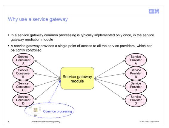
This slide shows a configuration that uses a service gateway. When a service gateway is used, you need to implement any common processing only once, in the service gateway mediation module. The mediation flow in the service gateway mediation module is used by all of the service consumers. The service gateway provides a single point of access to all of the service providers, which can be tightly controlled.
