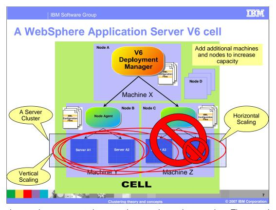
The nodes may be on separate boxes or they may be on the same box. They are shown here on separate boxes and the deployment manager is on a separate machine as well. To host more than one node, the host machine must have ample memory, disk space, and processor capacity.
