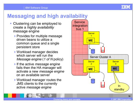
When an application server cluster is added as a member of the Service Integration Bus the Message Engine is created for the cluster using the active/standby pattern by default.
