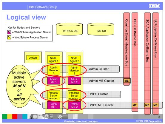
Notice the key in the upper left. There are two different kinds of servers in each node. The three nodes, deployment manager, Node 1, and Node 2, are represented by the yellow rectangles.
