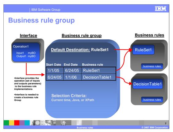
This graphic illustrates how a business rule group works. From left to right an Interface, which is an XML based WSDL file, provides the rule group with some inputs and outputs that will be used in a business rule. Again, the rule group needs an interface in order to work.
