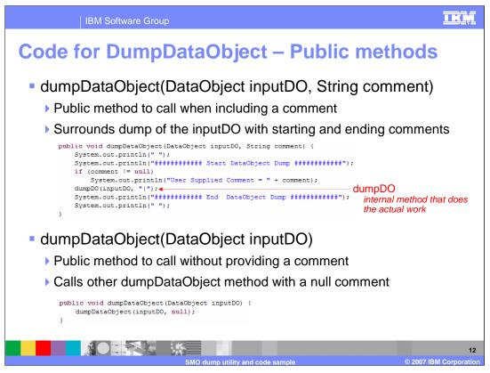
This slide shows the two public methods that can be called to do a DataObject dump. They are both called dumpDataObject and take a DataObject as input. The one on the top of the slide also takes a second parameter containing a comment to put into the dump.
