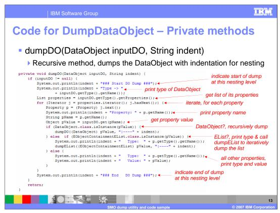
This slide shows the dumpDO method which does the real work for dumping a DataObject. As input it takes the DataObject to dump and an indentation string that is added to the front of each line of output. This enables the visual nesting of DataObjects when the routine is called recursively to dump DataObjects within DataObjects.
