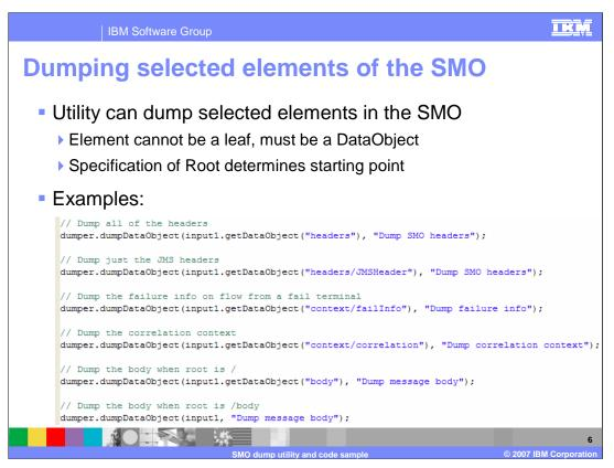
The utility is able to dump any DataObject. Therefore, you do not need to dump the entire SMO when the Root property is / (slash) or the entire SMO body when the Root is /body. Any element of the SMO can be dumped provided it is a DataObject rather than a leaf element.
