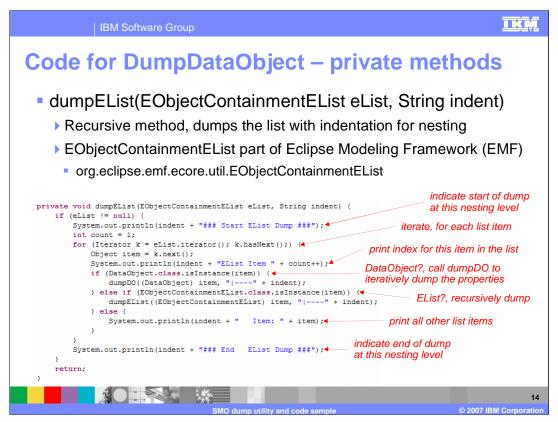
The method on this slide is used to dump an EList, or more specifically an EObjectContainmentEList. Similar to the dumpDO routine, it can be called recursively to handle an EList within an EList. It also has support for the indentation string, allowing the output to have a visual indication of the nesting.
