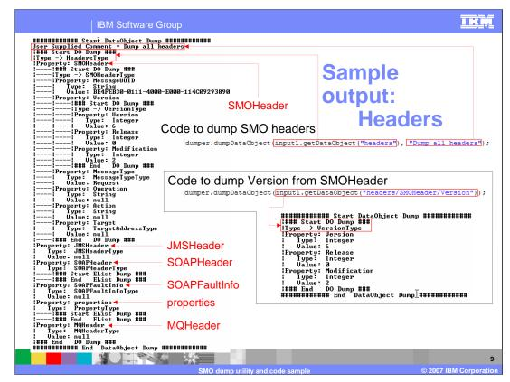
There are two examples on this slide, one for the entire headers section of the SMO and the other for the Version contained within the SMOHeader. Both of these examples require that the root be specified as / (slash).
