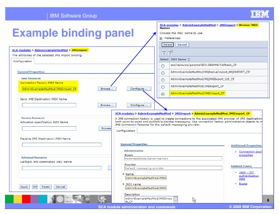
By clicking on the JMS imports from the previous panel, the configuration of the JMS provider can be modified. The browse button allows selection of the JNDI name to be used. The configuration button allows the selected JNDI provider to be viewed and modified.
