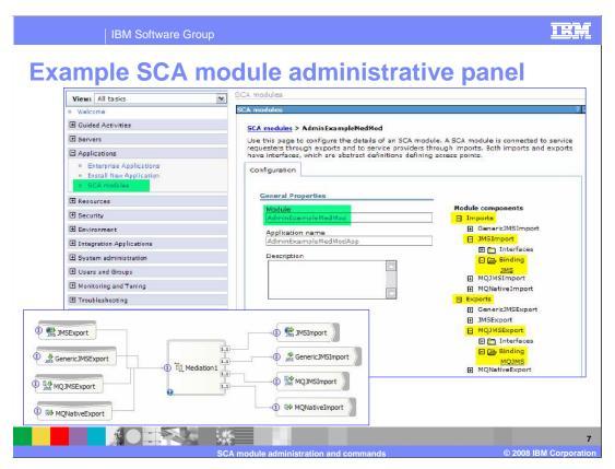
In the details of the module, the imports and exports can be seen. These views represent the bindings that were selected during the creation of an SCA module within WebSphere Integration Developer.
