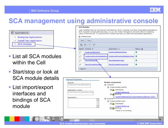
SCA modules are exposed within the Application group. Clicking on the SCA module, you can start or stop the module, or look at the details of the module.
