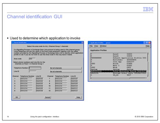
The last option in the pack configuration GUI is the Channel Identification setting. The screen captures show a default configuration for a channel group consisting of 12 channels and a set of application profiles that are available.
