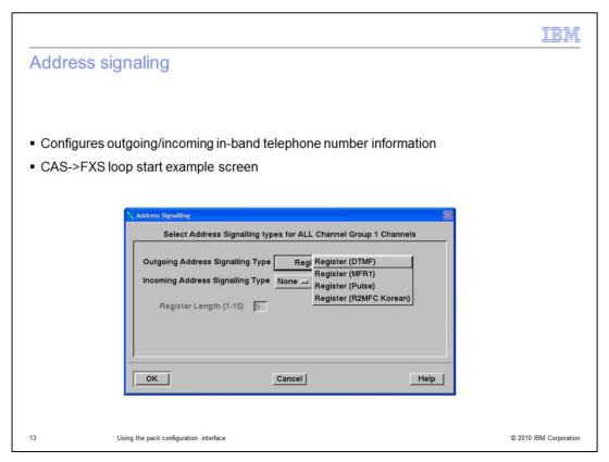
This screen is displayed when you click the Address Signaling button on the Pack Configuration GUI.
