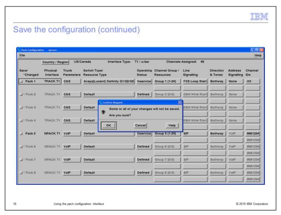
Once the parameters have been saved, you can close the Pack Configuration GUI by clicking File->Close and then clicking OK on the Confirm Request dialog.
