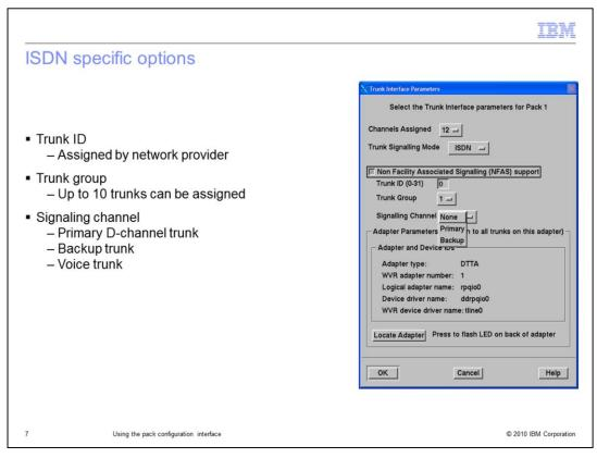
For T1 systems only, if you select ISDN for the Trunk Signaling mode then additional options are available as shown in the screen capture. It is not applicable to E1 systems.
