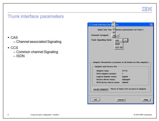
This screen is displayed when you click the Trunk Parameters button on the Pack Configuration GUI.
