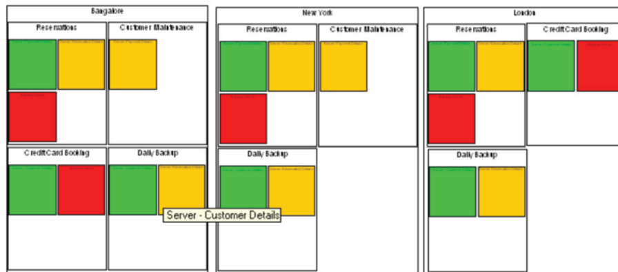
Figure 3: Screenshot of how Telelogic System Architect software can help organizations compare power usage between locations, divisions or departments. This screenshot shows server power consumption among systems in three different locations using colors: green (low), amber (medium) and red (high).
