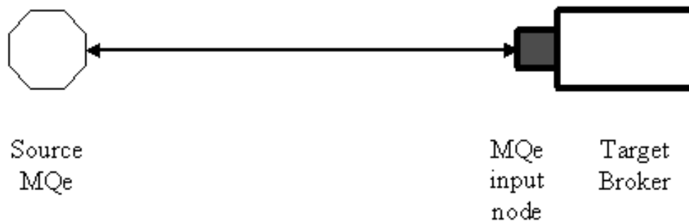
Figure 4. Publish/subscribe via the MQe broker input node
