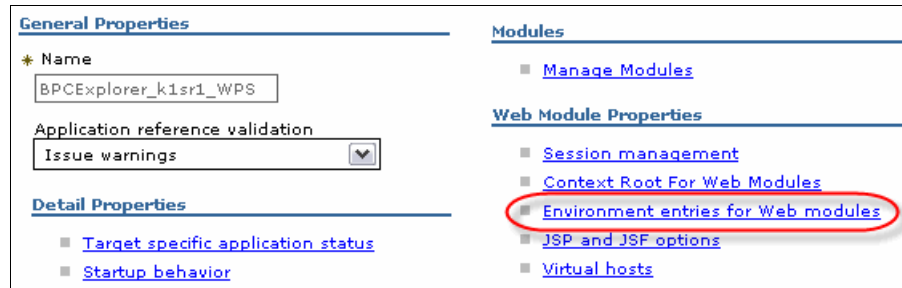
Figure 8-5 Click Environment Entries for Web Modules in order to change the REST URL:port
