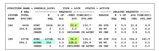
The decision is continuously reevaluated by allowing every nth SYNC request to be issued unchanged and comparing it with the thresholds.
