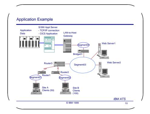
An example application will to used to show how to apply the steps for measuring availability. It uses a e the infrastructure supporting of the most common and growing applications today - the "web-enabled" or "e-business" application. These applications allows end users on the intranet or internet to access functions and information in "legacy" applications via web connections.
