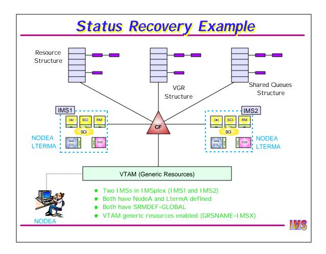
We are going to walk through an example of STM Global status recovery. This diagram shows two IMSs (IMS1 and IMS2) which each have NODEA and LTERMA defined. These IMSs are part of a data sharing group, a shared queues group, and a VTAM generic resources group (GRSNAME=IMSX).
