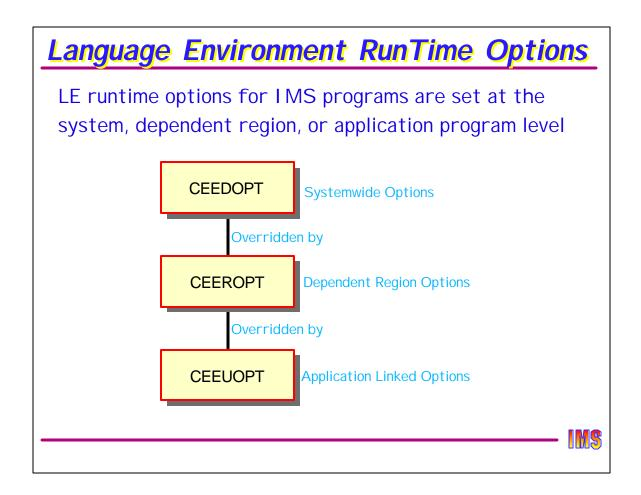
LE runtime options can be set at several levels, with each lower level overriding the higher levels. The levels are:
