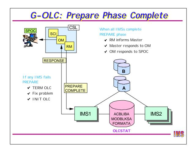
When RM gets a response from all IMSs, it notifies the Prepare Master who then notifies the operator that prepare is complete. If any IMS fails the prepare phase (for example, an I/O error on ACBLIB), then the operator must terminate OLC with the TERMINATE OLC command, fix the problem, and then repeat the process.
