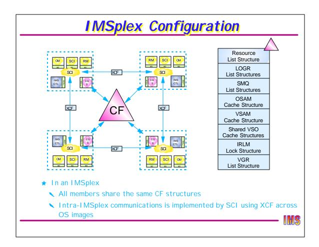
When there are multiple IMSs within the IMSplex, each IMS (actually each MVS image) must have a copy of the SCI address space. Only one copy of OM and RM is needed, although for availability and performance, it is recommended that several, or one per MVS image, be started. Wherever there is an IMS with shared queues, or an RM with a Resource Structure, there needs to be a CQS. Remember, one CQS can serve both the Shared Queue structures and the Resource structure.
