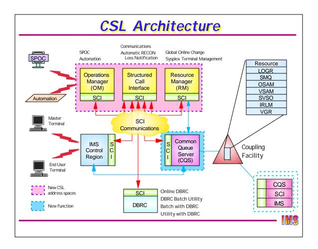
This is a diagram of the CSL architecture showing the new address spaces and the new resource structure. There may be (probably are) additional images on other LPARs. All CSL address spaces communicate using SCI.
