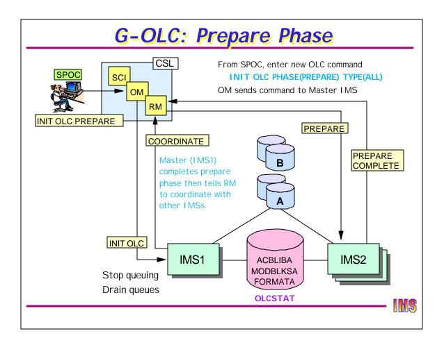
In a bit more detail now, when the PREPARE command is entered, OM sends the command to one of the IMSs in the G-OLC to be the PREPARE MASTER. That IMS will perform the prepare phase locally and, if successful locally, tells RM to coordinate the prepare phase across the other IMSs. As each IMS completes its prepare processing, it notifies RM.
