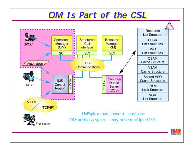
This chart shows the IMSplex components with interfaces to OM. Not shown is that the Resource Manager also registers with OM for one command (QUERY STRUCTURE). The SPOC (Single Point of Control) is used to describe any OM client where a human operator enters commands. The automation symbol indicates any program which enters commands without human intervention, such as a NetView EXEC.
