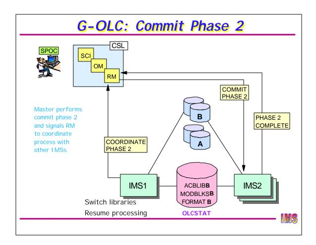
Once the OLCSTAT data set updates are complete, the master signals RM to coordinate Commit Phase 2 with the other IMSs. During this phase, the IMSs switch libraries and resume processing. When this is done, they signal Phase 2 complete. If any IMS fails Commit Phase 2, a return code and reason code explain why and the problem must be corrected and the commit command reentered. Phase 3 cannot begin until all IMSs have completed Phase 2.
