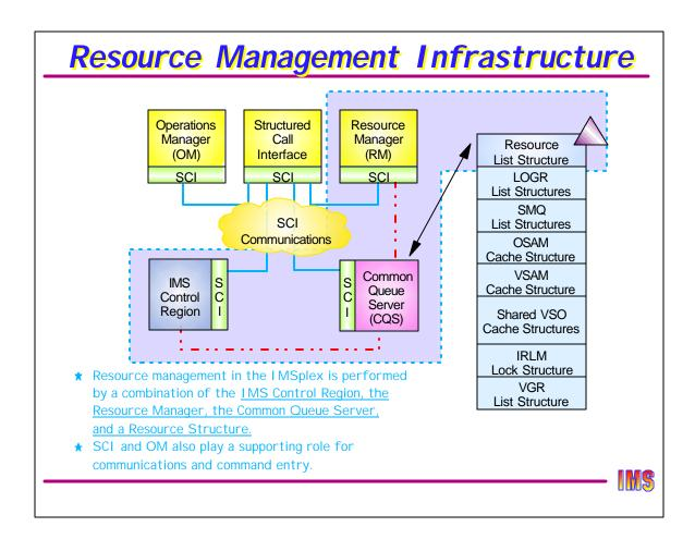
The complete architecture of Resource Management in the IMSplex is shown here. Full service requires an IMS control region, a Resource Manager, the Common Queue Server, and a Resource Structure. If no resource structure is defined, then CQS is not required (unless, of course, shared queues is active).
