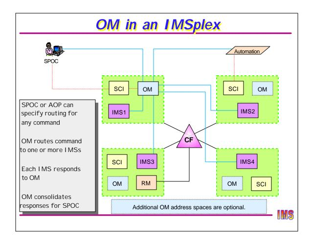
This chart shows (at a high level) the flow of processing when an OM client enters a command to IMS and gets a response. The client must first register with SCI. SCI must be on the same MVS image as the client.
