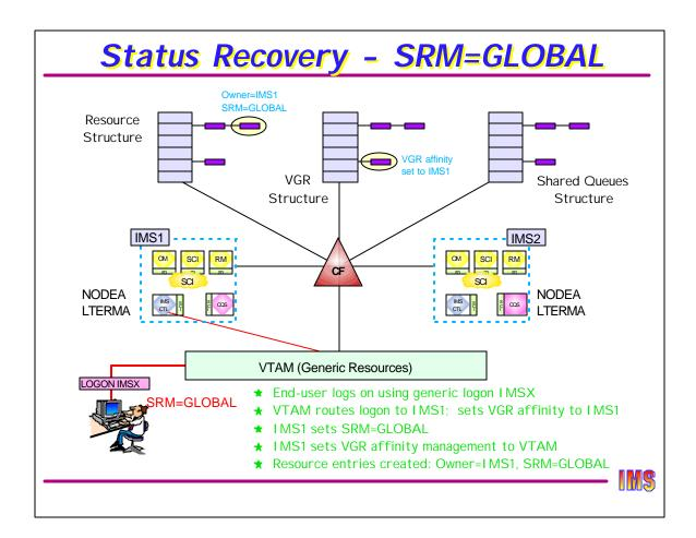
A user logs on from NodeA using the generic resource name IMSX. VTAM will check the VGR structure and determine that this node does not currently have an affinity for any application in the IMSX generic resource group. It selects one of the active IMSs to route the logon request to. In this example, it is IMS1.
