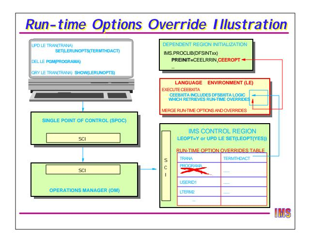
This diagram follows the logic (at a high level) when the TERMTHDACT option is set for TRANA. IMS must be enabled for this capability by having LEOPT=Y or setting it on with the UPD LE command.
