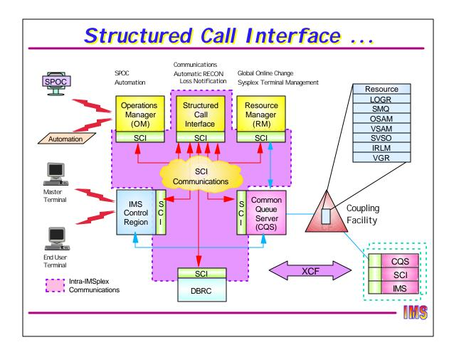
This shart just shows that SCI is involved with every member. Each individual member has an SCI interface which it invokes to register or communicate with other members. When communications is with a member on another MVS image, then XCF signalling services are used to send the message.
