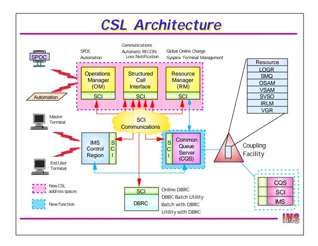
This diagram shows a minimum configuration for IMS in a CSL environment utilizing all functions. The three new address spaces are shown with the function they support written above them. For example, OM supports SPOC and Automation.
