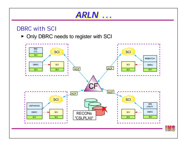
This is an illustration of the use of SCI by DBRC. Each DBRC instance in an IMSplex shares the same set of RECONs. The IMSplex name is stored in the RECONs. Each DBRC instance registers with SCI. It uses the IMSplex name for the registration. SCI is used for communication between the DBRCs in an IMSplex. SCI uses XCF for communication between different LPARs.
