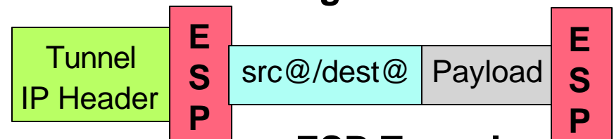
ESP-Tunnel (hides endpoint addrs)
