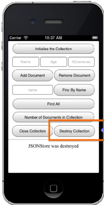
Destroy the internal storage associated with a collection and clear the keychain that stores necessary keys for decrypting the internal storage.
