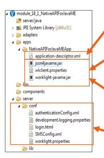
The **application-descriptor.xml** file is used to define the application metadata and to configure the security settings to be enforced by Worklight Server.
