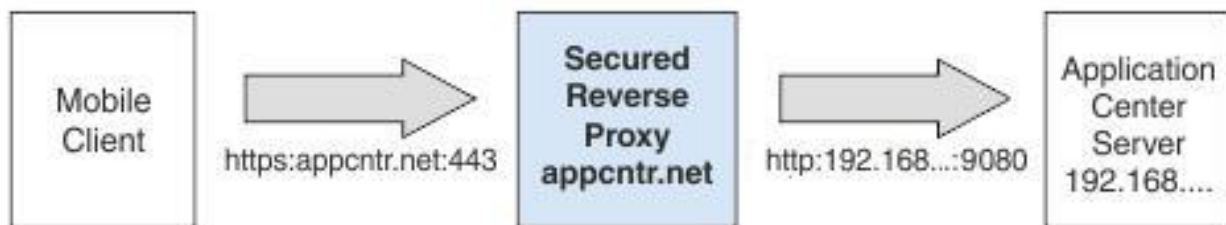
Figure 11. Configuration with secured reverse proxy
