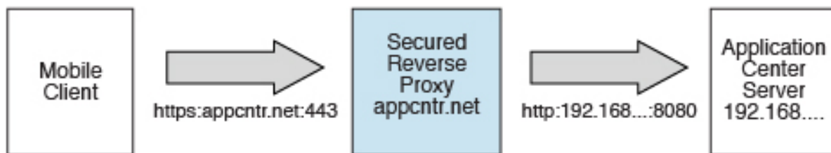
Figure 6-15. Configuration with secured reverse proxy
