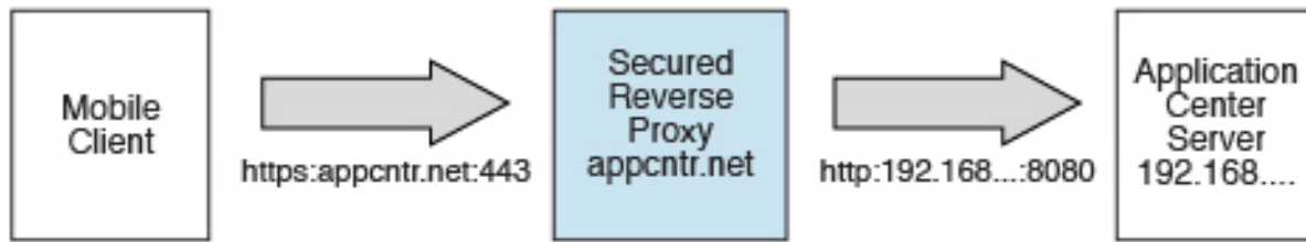
Figure 6-12. Configuration with secured reverse proxy
