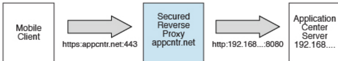
Figure 6-19. Configuration with secured reverse proxy
